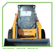
**OVER-THE-TIRE** design provides wider access and improved visibility. *Models 2200R and 2600R*
